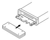
Note that if the front panel fails to lock in position properly, pressing control button may not function and display may be missing some segments.Press the OPEN button and then reinstall the front panel again.
